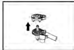
3. Unscrew the motor cover.
