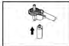
6. Install the new motor.
