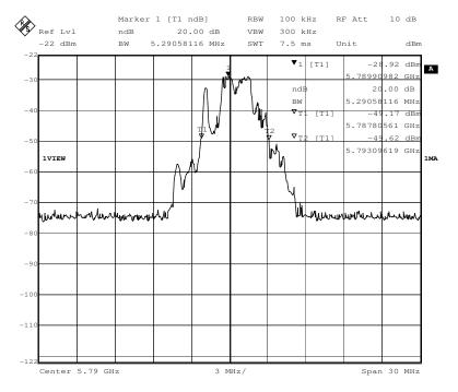
After a more accurate measurement, the occupied bandwidth revises to 5.29058116MHz.
