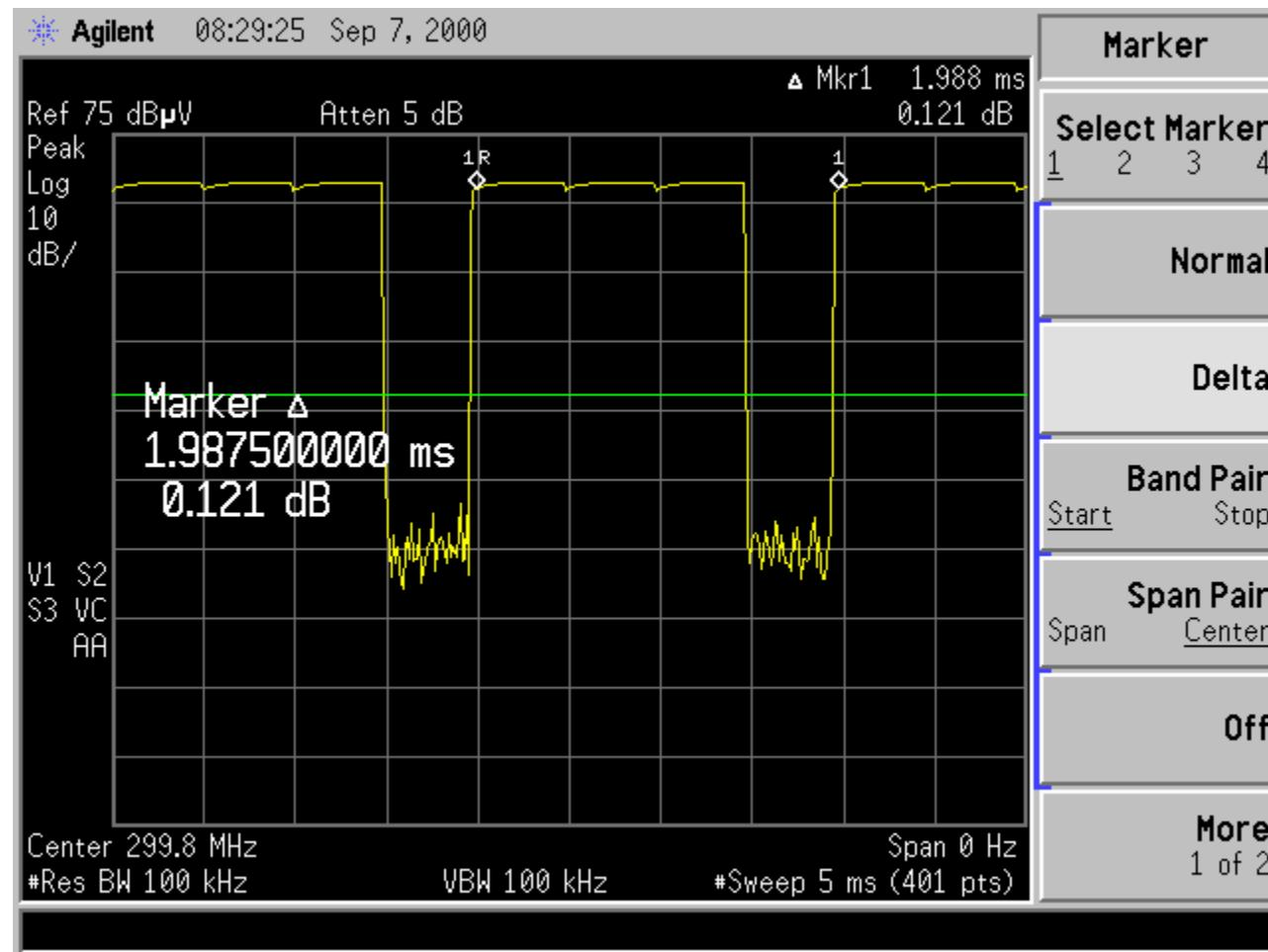
**Transmitter Turn-Off Release Time, Upon Momentary Activation of Push Switch
