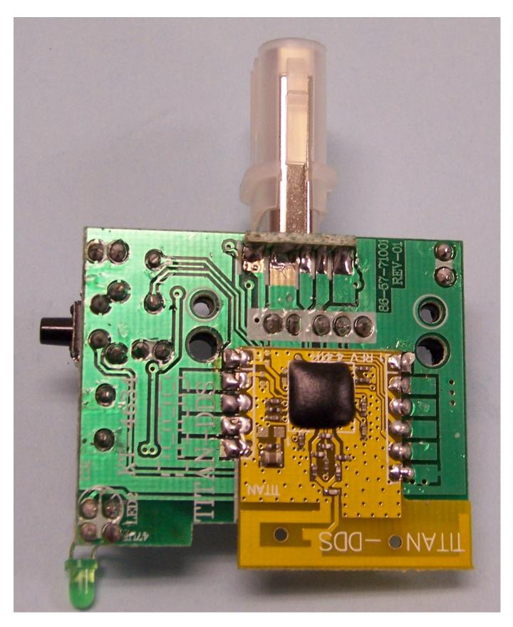
Note: Radio Card lies flat upon the functional PCB. There are no components underneath.
