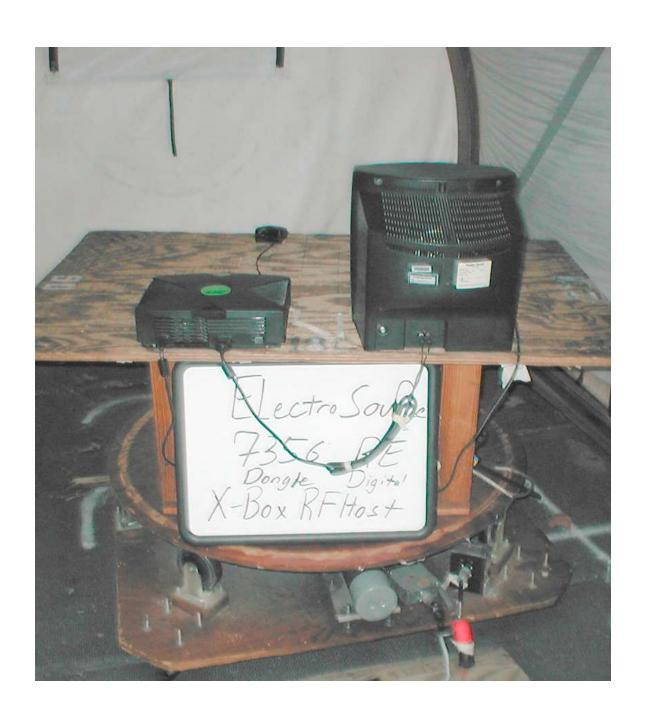
**Conducted Emissions Test Setup**
