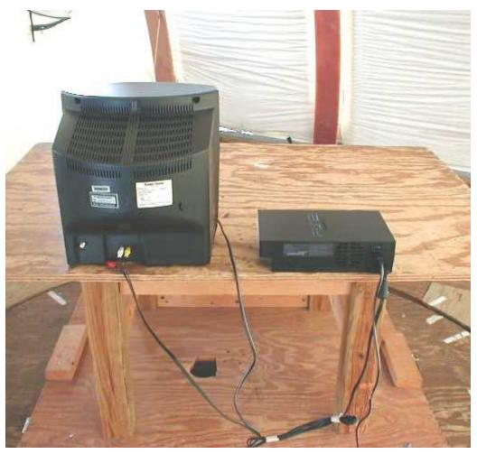
**Conducted Emissions Test Setup**
