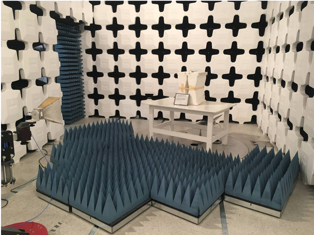
Figure 2. Intentional Radiated Emissions Test Setup, Above 1GHz
