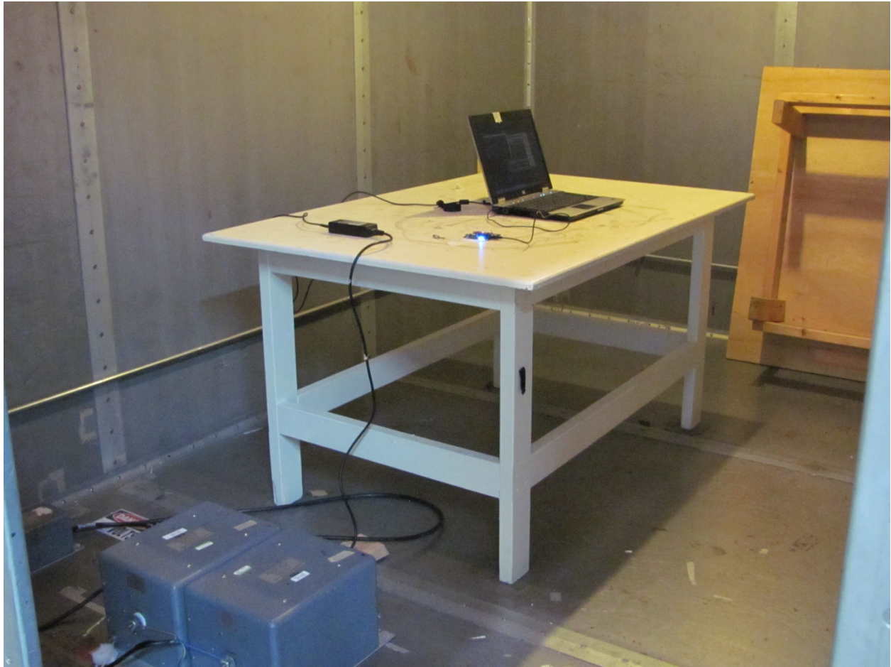
Figure 9. Power Line Conducted Emissions Test Configuration Photo
