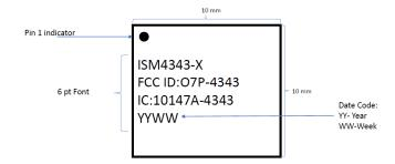
Label will be stamped onto the 10x10mm ISM4343-WBM-L151 Chip
