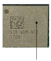
Label will be stamped onto the 10x10mm Chip
