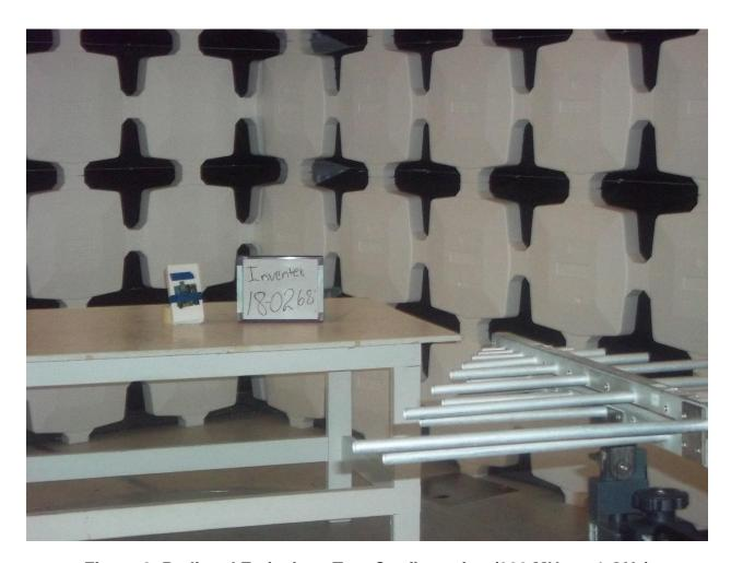
Figure 3. Radiated Emissions Test Configuration (200 MHz to 1 GHz)
