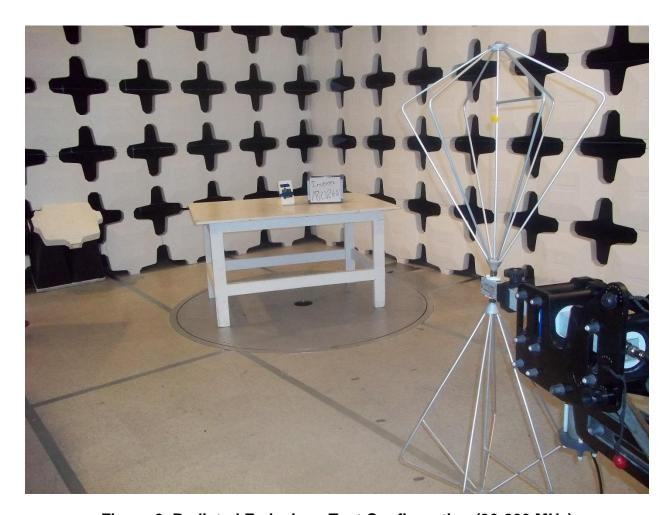
Figure 2. Radiated Emissions Test Configuration (30-200 MHz)
