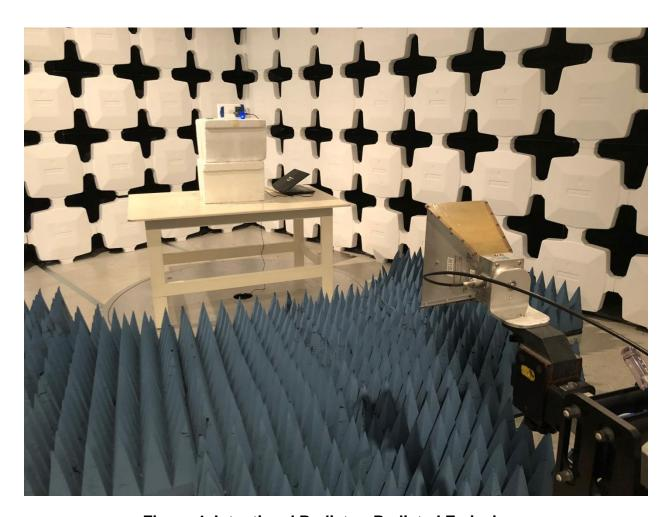
Figure 4. Intentional Radiator, Radiated Emissions
