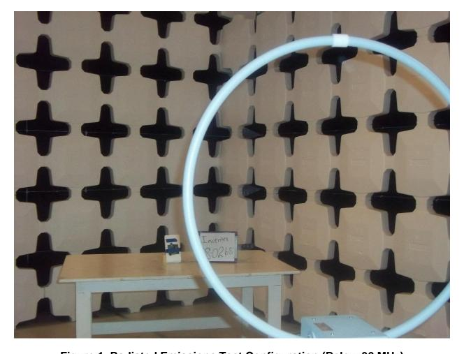
Figure 1. Radiated Emissions Test Configuration (Below 30 MHz)
