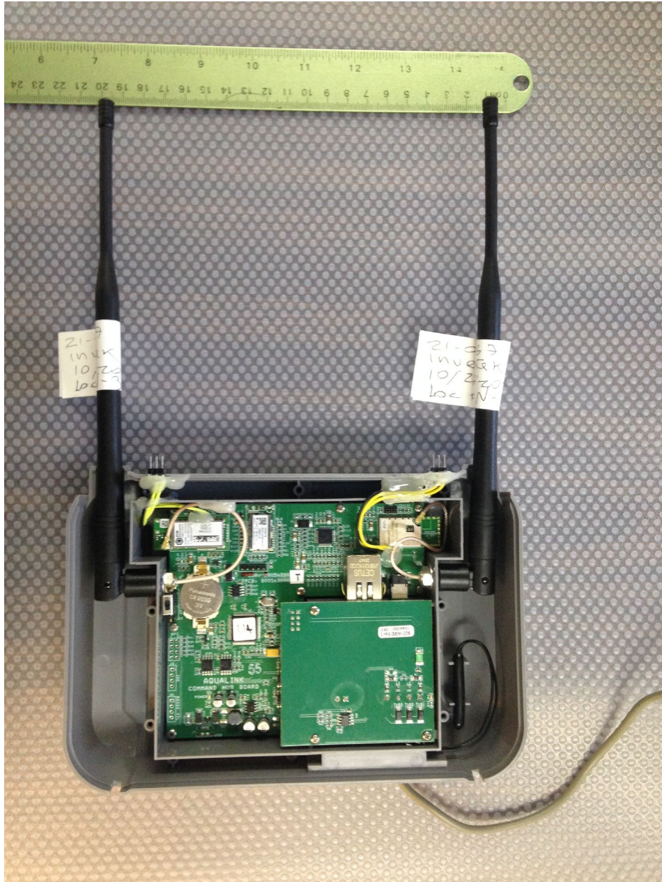
Figure 1. Antenna Elements within 20cm of each other
