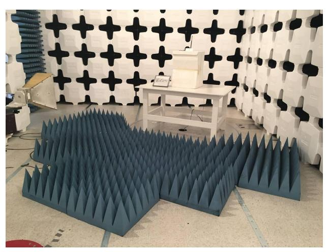
Figure 2. Intentional Radiated Emissions Fundamental and Harmonics Testing
