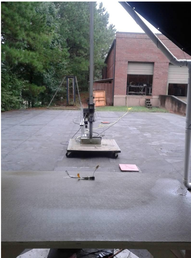
Figure 5. Radiated Emissions Test Setup using Module with WiFi+BT+NFC 200 MHz to 1GHz
