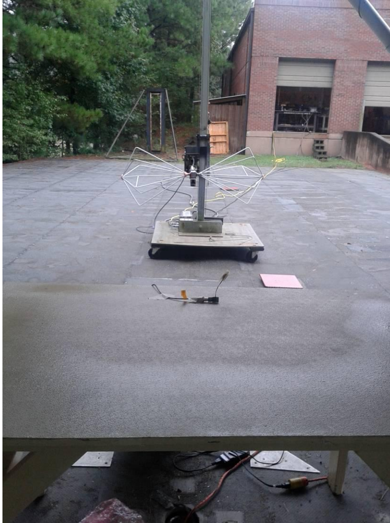
Figure 4. Radiated Emissions Test Setup using Module with WiFi+BT+NFC 30 MHz to 200 MHz, Back
