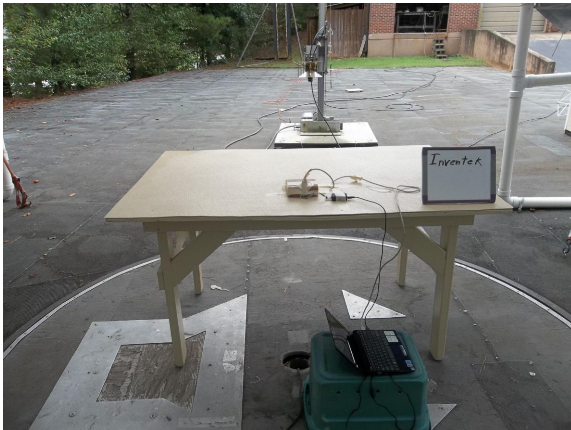
Photo 6. Radiated Emission Test Setup, above 1 GHz, Rear view
