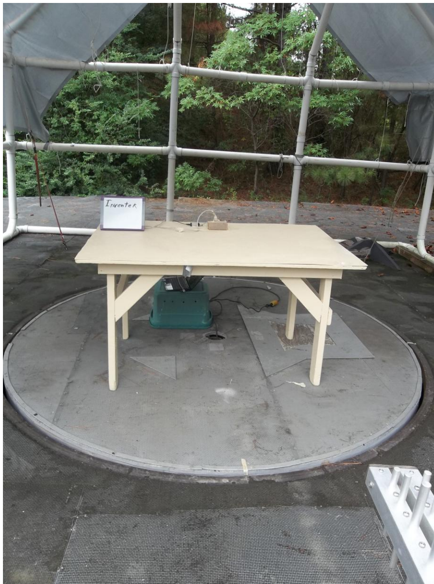
Photo 2. Radiated Emissions Test Setup, Front View
