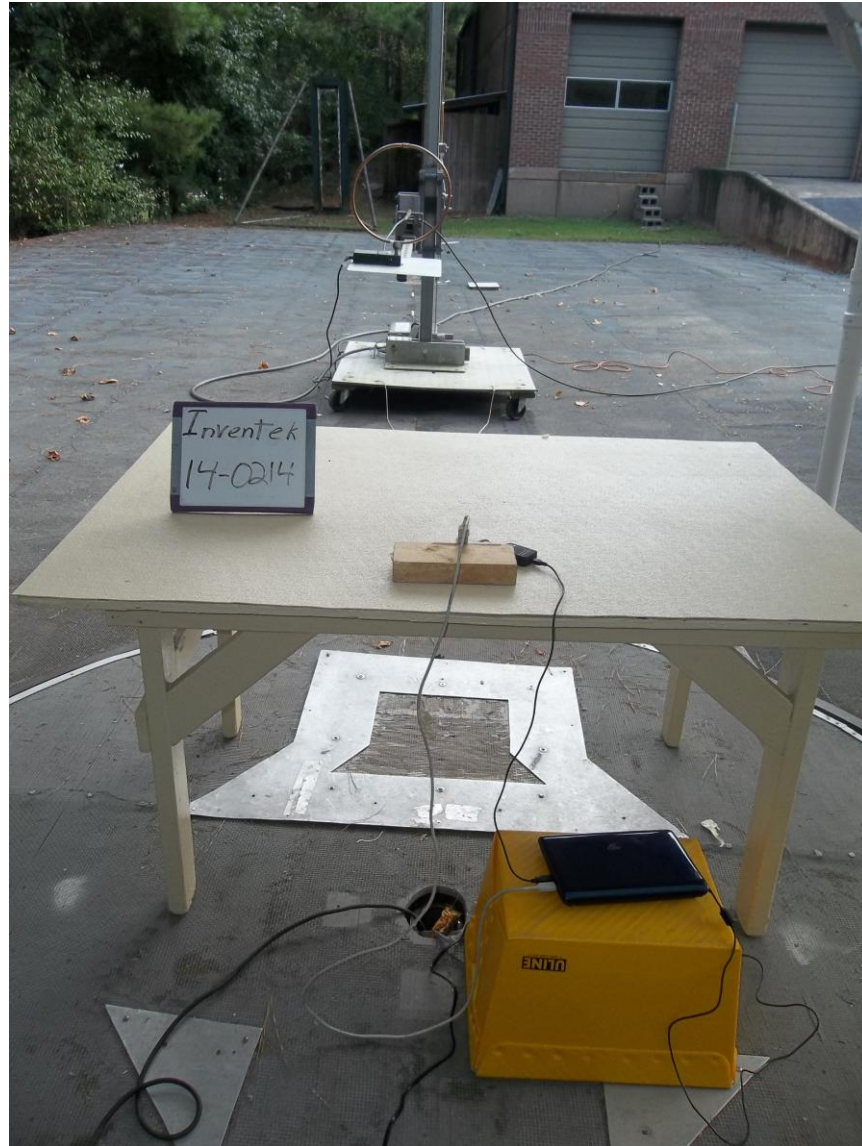
Photo 3. Radiated Emissions Test Setup, 0.15 MHz to 30 MHz, Rear View
