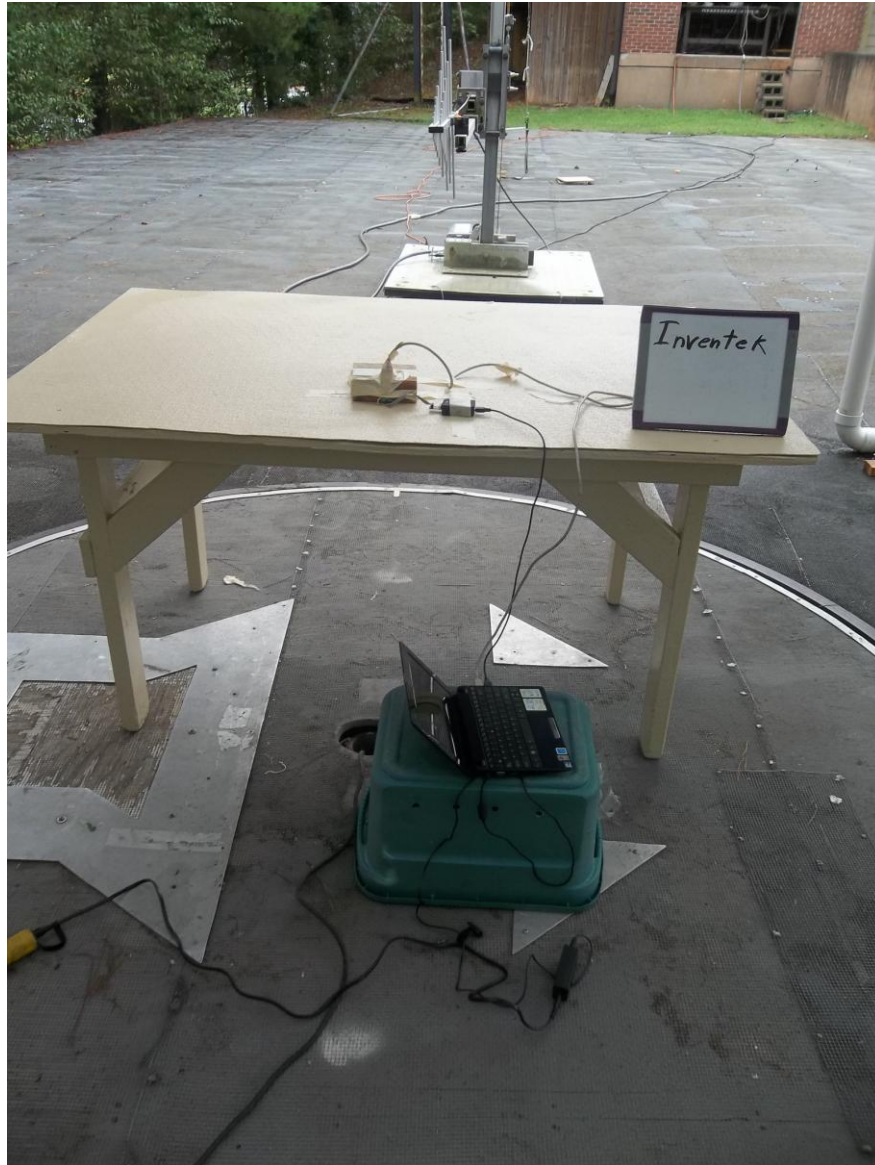
Photo 5. Radiated Emissions Test Setup, 200 MHz to 1GHz, Rear View
