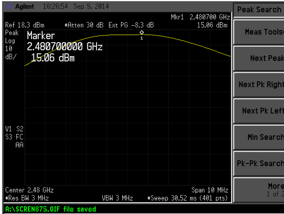
Figure 24. Peak Antenna Conducted Output Power, High Channel
