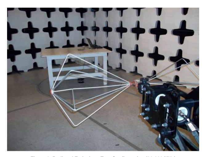
Figure 3. Radiated Emissions Test Configuration (30-200 MHz)
