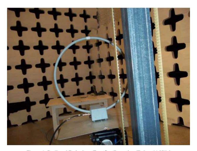
Figure 2. Radiated Emissions Test Configuration (Below 30 MHz)
