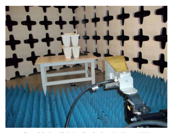
Figure 5. Radiated Emissions Test Configuration (Above 1 GHz)
