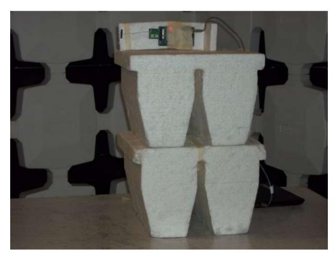
Figure 1. Radiated Emissions Test Configuration (above 1 GHz), Close-Up
