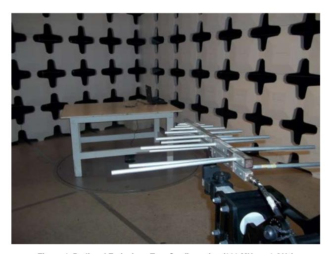
Figure 4. Radiated Emissions Test Configuration (200 MHz to 1 GHz)
