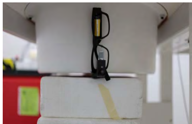
Fig.5 Position the inside of the arm against the phantom(Plot 3)
