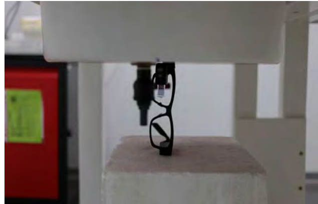
Fig.3 Position the outside of the arm against the phantom(Plot 1)
