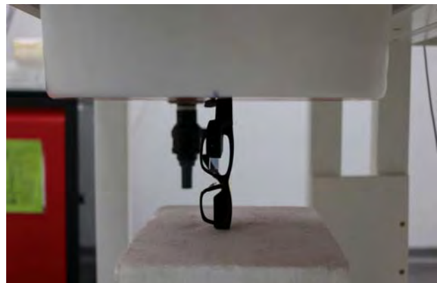
Fig.4 Position the outside of the arm against the phantom(Plot 2)
