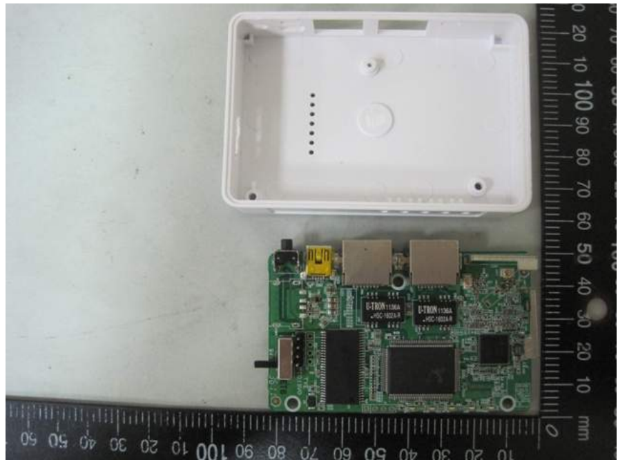
EUT 2. EUT with PIFA Antenna
