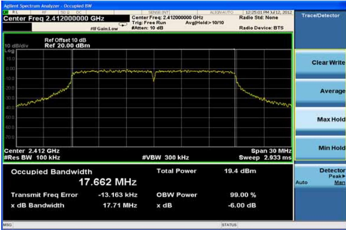
6dB Band Width Test Data CH-Mid
