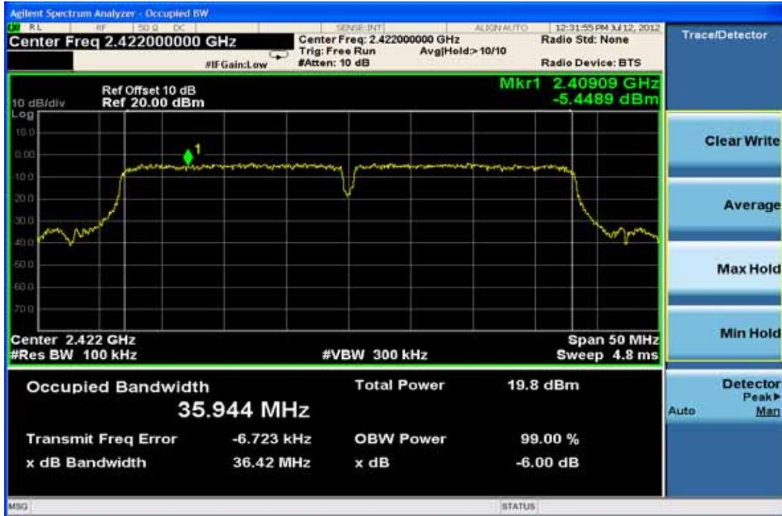
6dB Band Width Test Data CH-Mid
