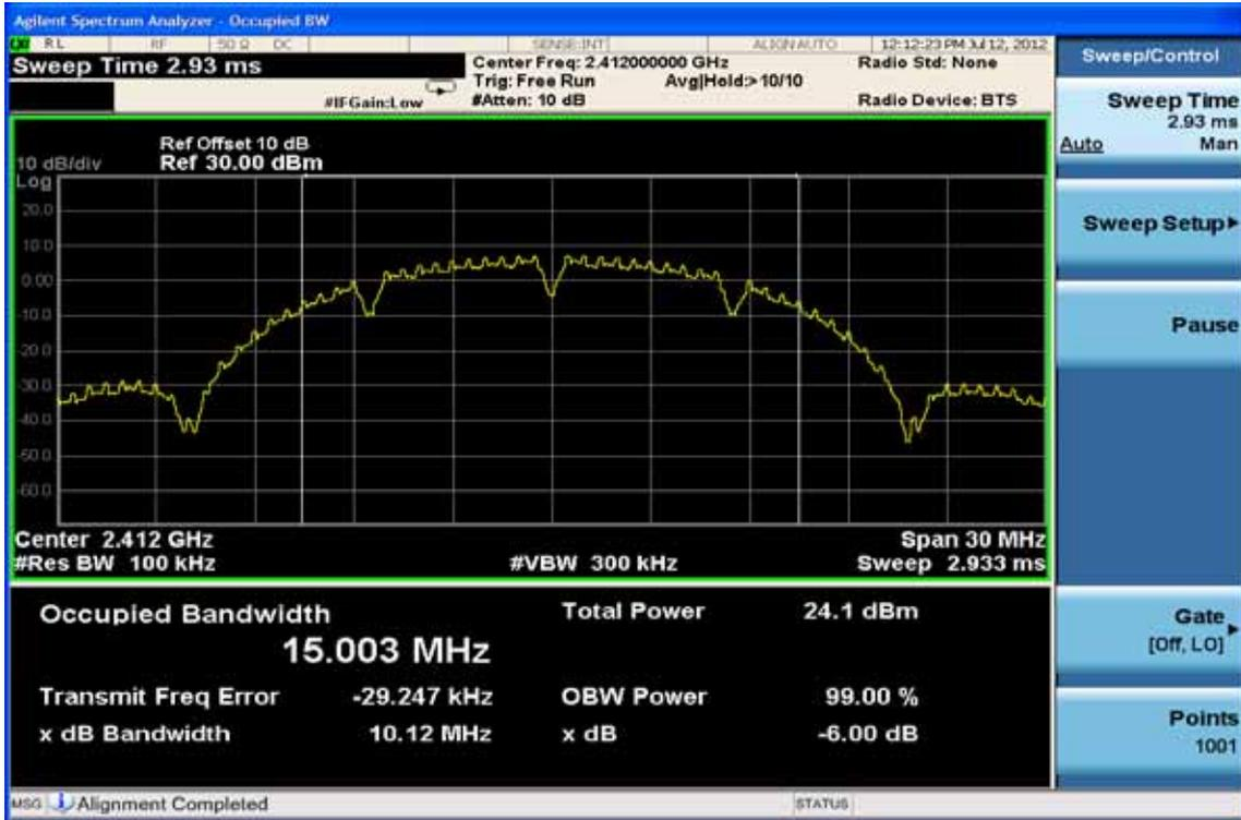
6dB Band Width Test Data CH-Mid
