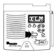
PTT / VOX - To Set the PTT / VOX sensitivity in the PTT position for manual push-to-talk transmissions or in the VOX mode for automatic voice-activated transmissions.
