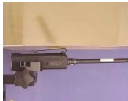
Body-worn SAR Test Setup 1.2cm Belt-Clip Separation Distance
