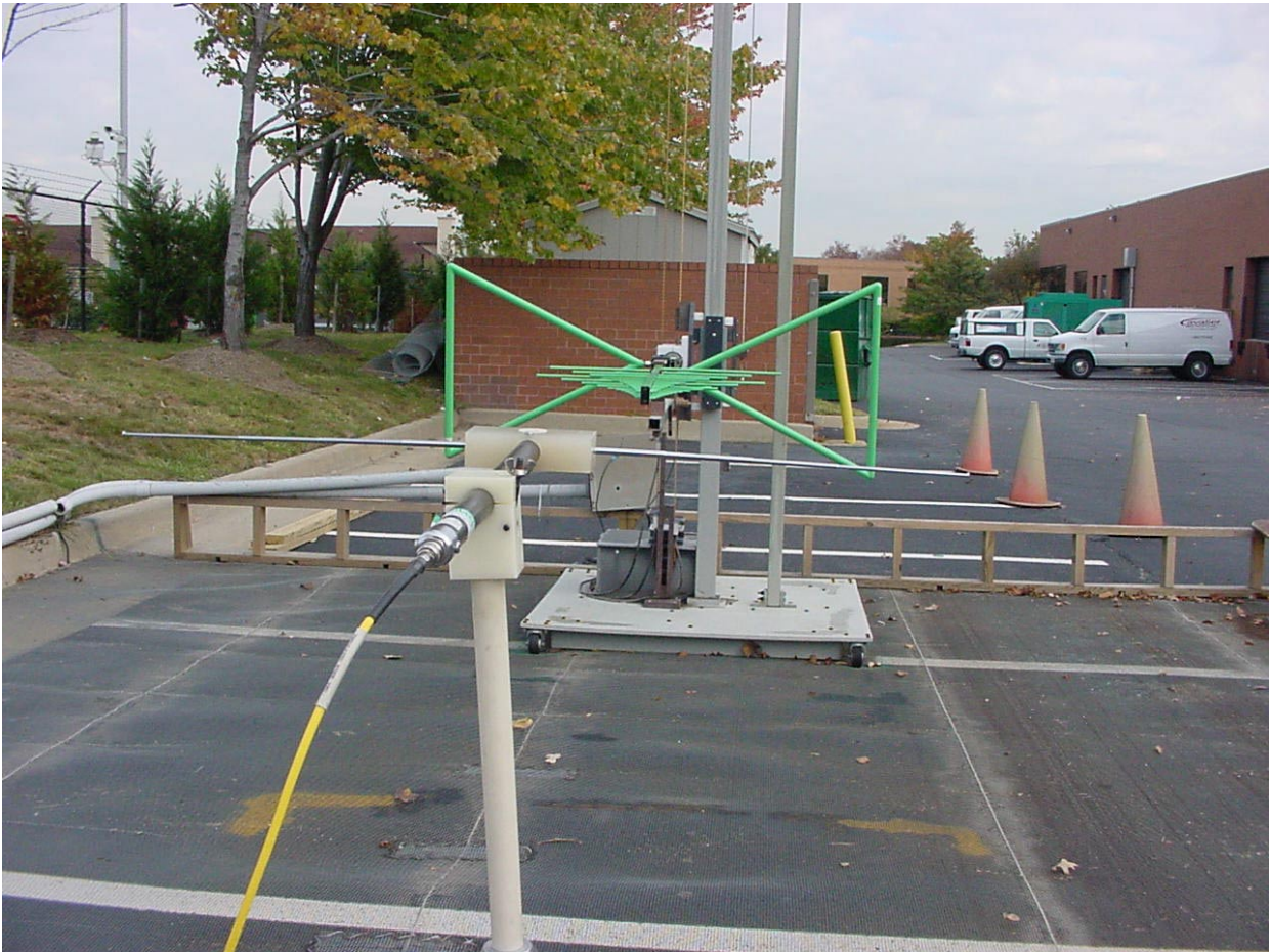
PHOTOGRAPH 5: SUBSTITUTION TRANSMITTING DIPOLE ANTENNA USED FOR FREQUENCIES (30 MHz – 1 GHz)
