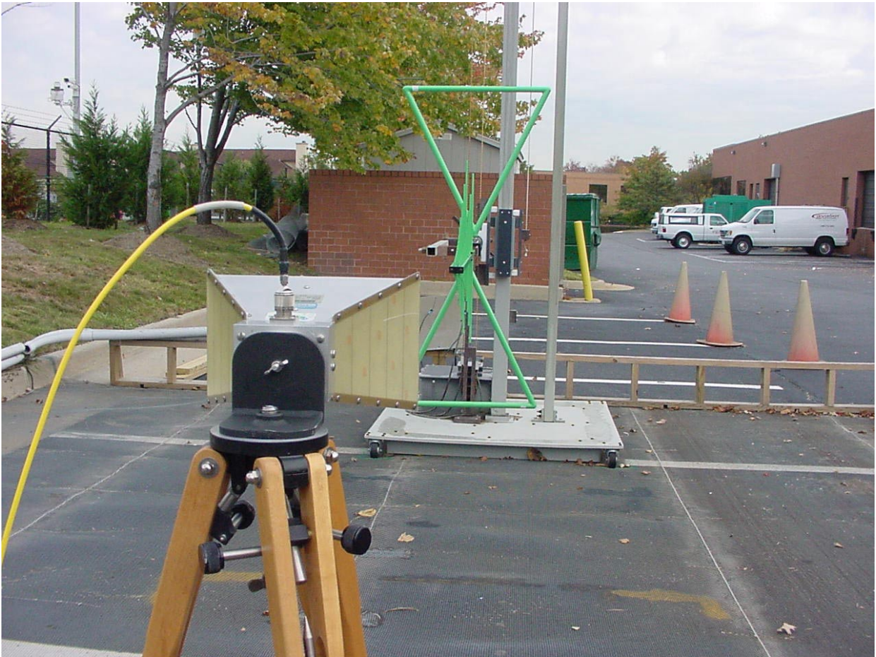
PHOTOGRAPH 6: SUBSTITUTION TRANSMITTING HORN ANTENNA USED FOR FREQUENCIES (1 GHz-18 GHz)
