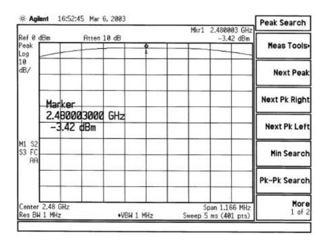
At the 2480 Mhz, The measured output power is -3.42 dbm.
