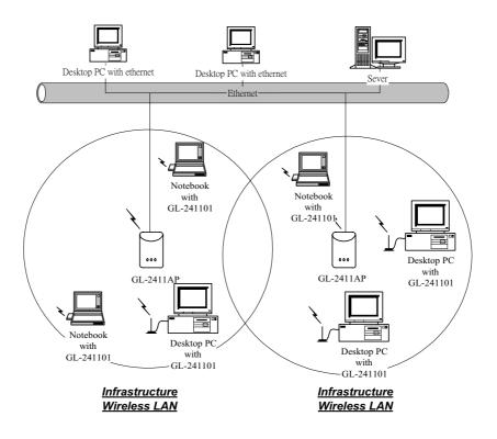
Fig. 2 - Infrastructure Wireless LAN Configuration
