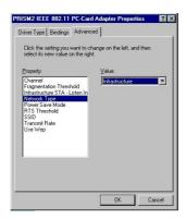
**Note**: "Infrastructure" mode allows a wireless adapter to communicate with a wired network, while "Ad-Hoc" mode allows wireless-to-wireless communication. Consult your System Administrator for information about your network communication type. For more information about Infrastructure and Ad-Hoc networks, see Chapter 2 of this manual
