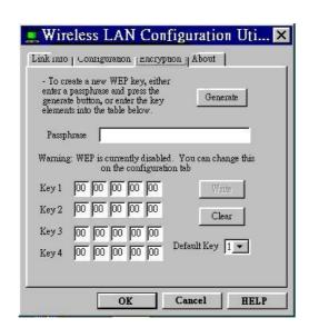
The 40-bit WEP keys can be generated from a user-defined passphrase (any text string with a maximum of 32 characters). To generate encryption keys for each client communicating in the wireless network, complete the following steps:
