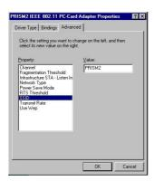
**NOTE**: The SSID can have any value, but should have the same value as the Access Point (AP). In Ad-Hoc mode, all clients should share the same SSID.
