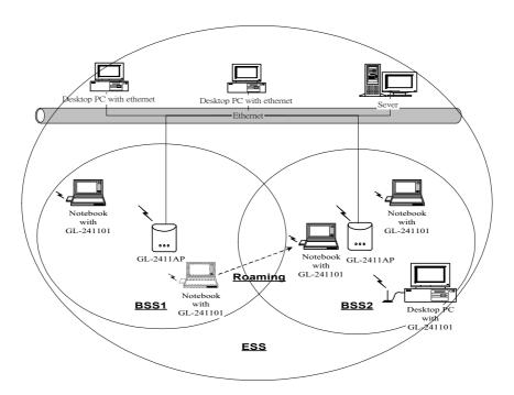
Fig. 4 - Roaming in an Extended Service Set (ESS)
