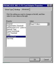
**NOTE**: Fixed 11 Mb/s is the preferred "Value" for environments where the client has line of sight access and is a short distance away from the AP. Fully Auto is the recommended setting for clients that are farther away from the AP and where there may be interference between the client and the AP.
