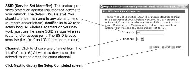
**CAUTION:** SSID and Channel number must be identical in all wireless network devices.
