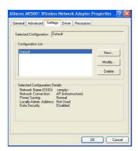
Atheros supports two encryption types; Wired Equivalent Privacy (WEP) and Advanced Encryption Security (AES). By default, the STA is set to auto and will first attempt to use AES and will only use WEP if AP only supports, or is configured for WEP only.
