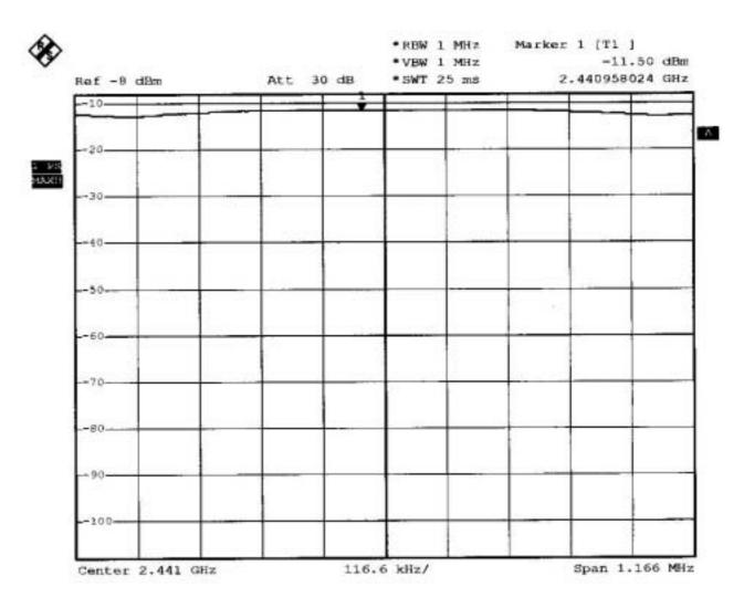
The Power (ERP) = Output power + cable loss + antenna gain = -11.50 dbm + 7.4 db + 1.9 dBi = -2.2 dbm
