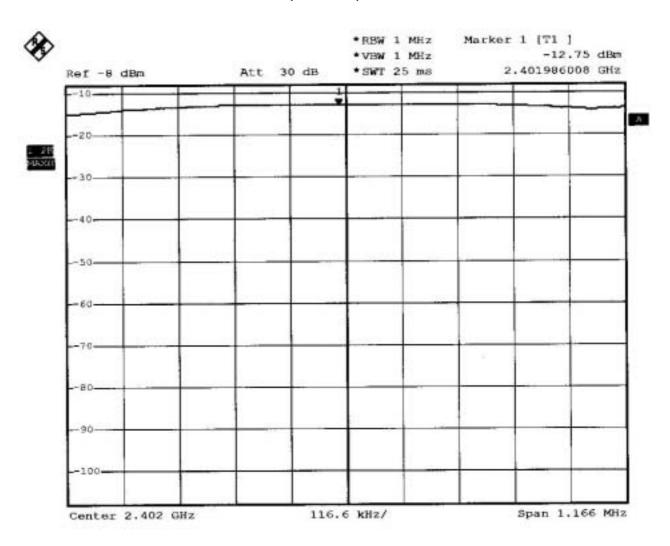
The Power (ERP) = Output power + cable loss + antenna gain = -12.75 dbm + 7.4 db + 1.9 dBi = -3.45 dbm
