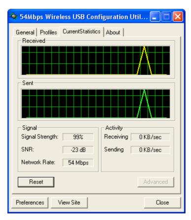
This screen graphically displays the received and sent traffic rates of the wireless USB adapter. The graphs sample time is definable by users in the preference option.
