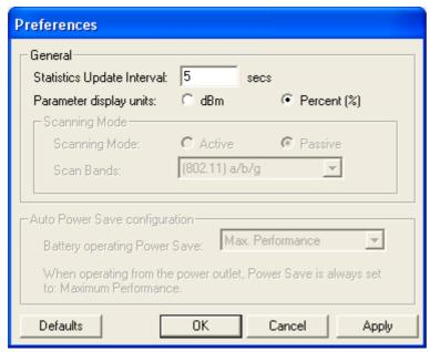
Statistic Update Interval: the sample rate in secs of the throughput.
