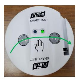
4. Use your hand to wave at the device from right to left (←) according to the table below. Confirm that the "blue" LED turns on.
