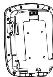
Step 3: Fix two M5 screws to complete the installation.
