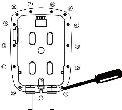
Step 2: Insert the SIM card according to the picture's instruction (for 4G Version).
