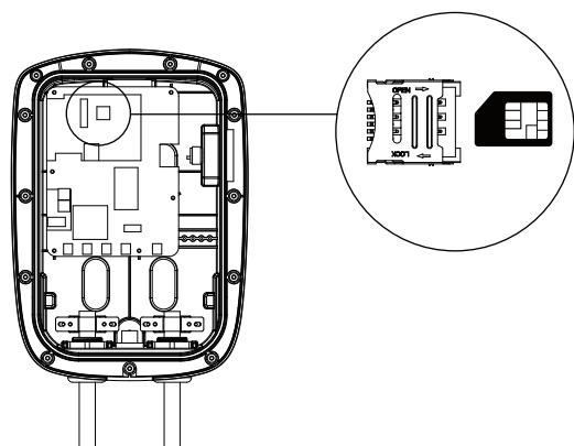
Step 3: Tighten 13 screws on the front cover after the front cover is put back, the recommended screw torque is 1.0 N.m (9.6 lbf.in) (for 4G Version).
