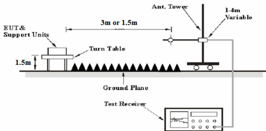
The radiated emission tests were performed in the 3 meters chamber test site, using the setup accordance with the ANSI C63.10-2013. The specification used was the FCC 15.209, and FCC 15.407 limits.
