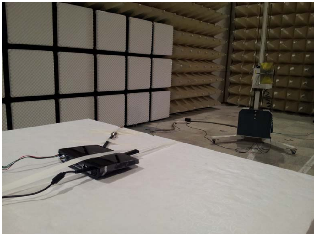
B. Photo of Radiated output power & Spurious Emission Test (BT)
