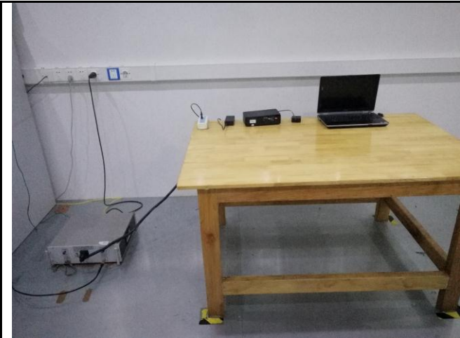
Conducted Emissions Test Setup Front View
