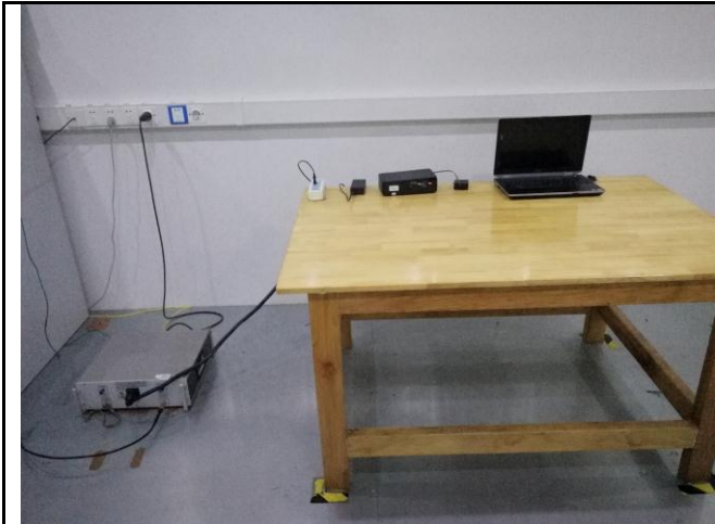
Conducted Emissions Test Setup Front View
