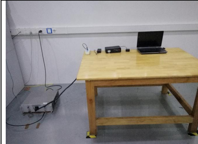
Conducted Emissions Test Setup Front View
