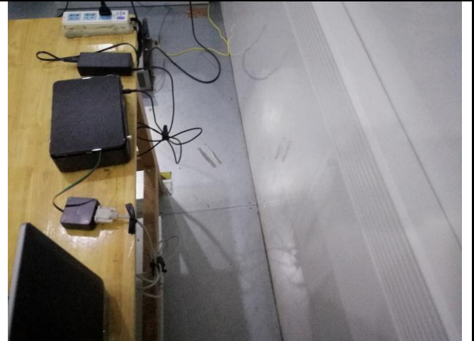
Conducted Emissions Test Setup Side View
