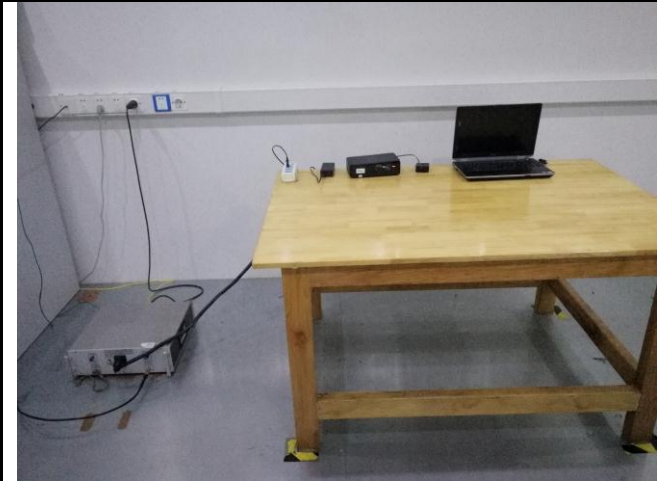
Conducted Emissions Test Setup Front View
