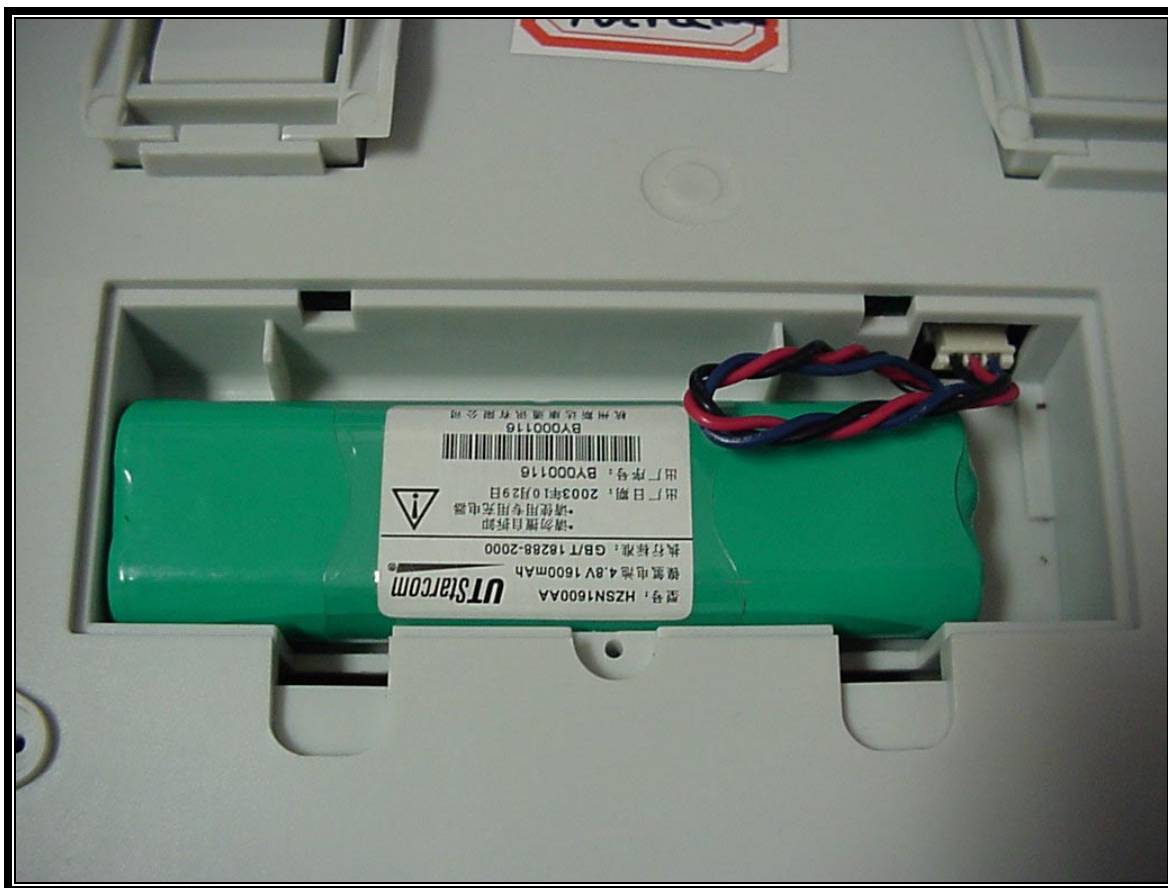
PHOTOGRAPH 43: BATTERY IN UNIT
