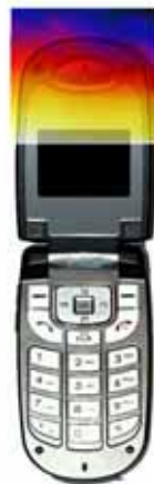
Figure 28 Sample H-field Scan Overlay
