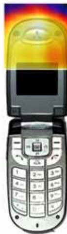
Figure 27 Sample E-field Scan Overlay
