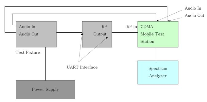
UART Interface: The UART Interface has a serial communication link that can be used to test, debug or upgrade the phone's functions and characteristics.
