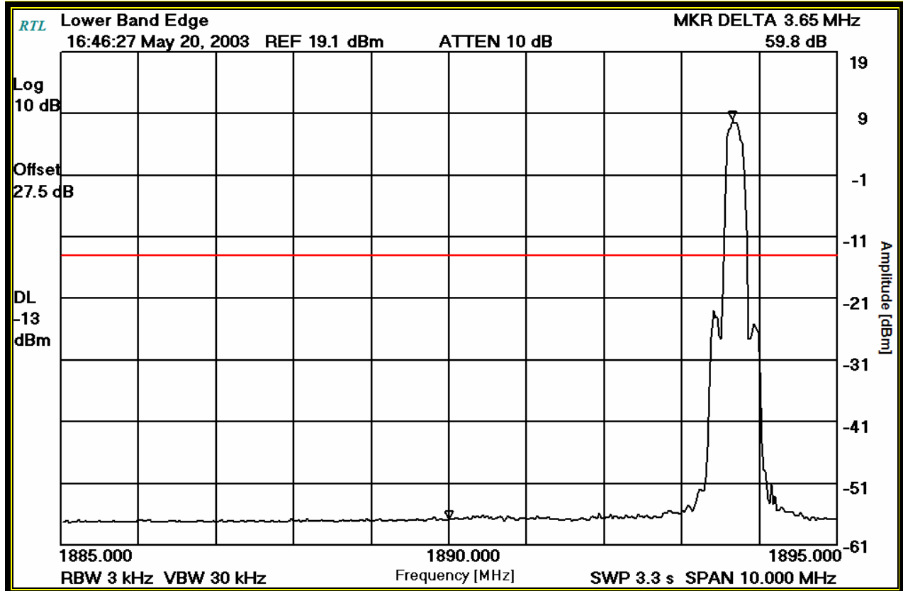
PLOT 8-1: LOWER BAND EDGE (LOWER BLOCK F)
