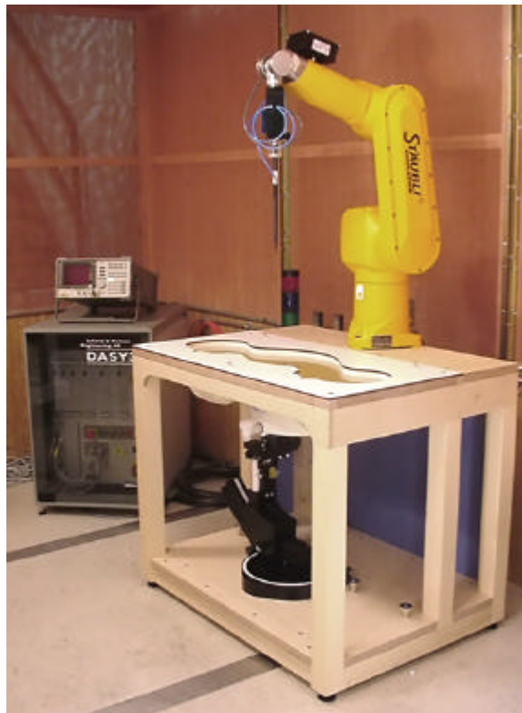
DASY3 SAR Measurement System with SAM Phantom
