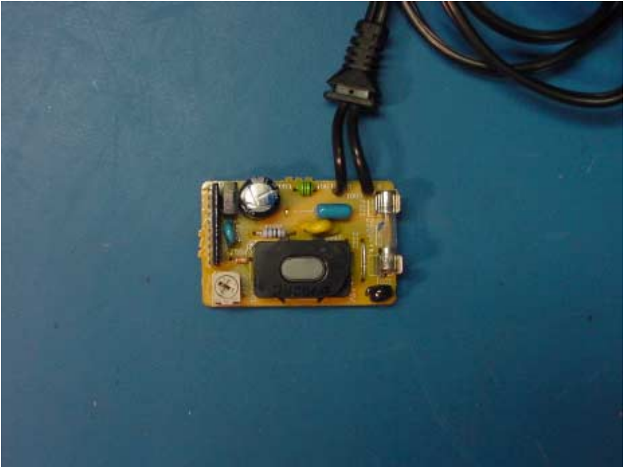
PHOTOGRAPH 16: RECHARGER MAIN TOP
