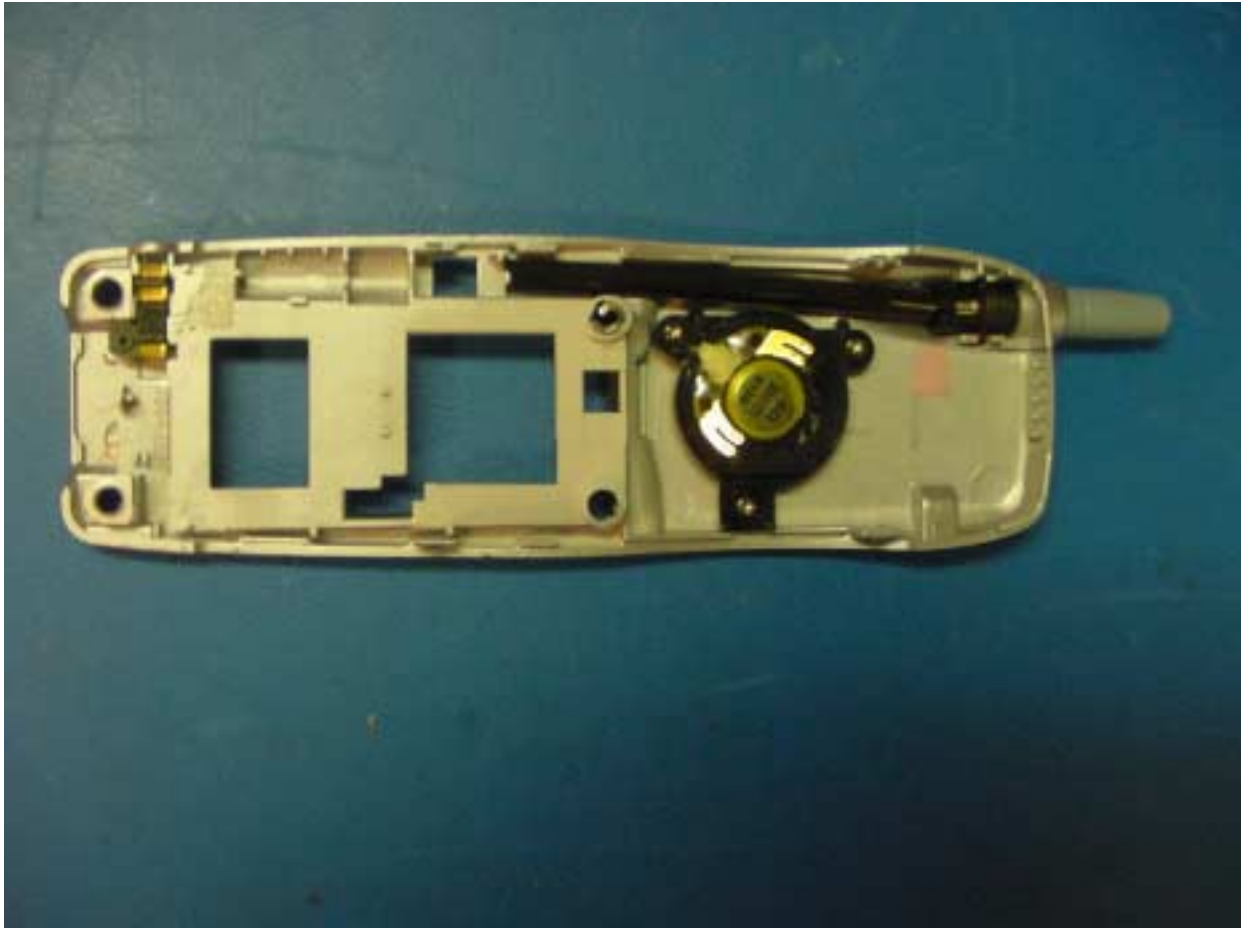
PHOTOGRAPH 7: INSIDE VIEW OF REAR COVER
