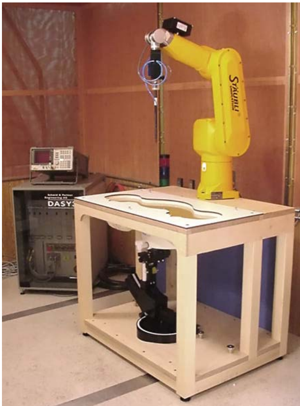
DASY3 SAR Measurement System with SAM Phantom
