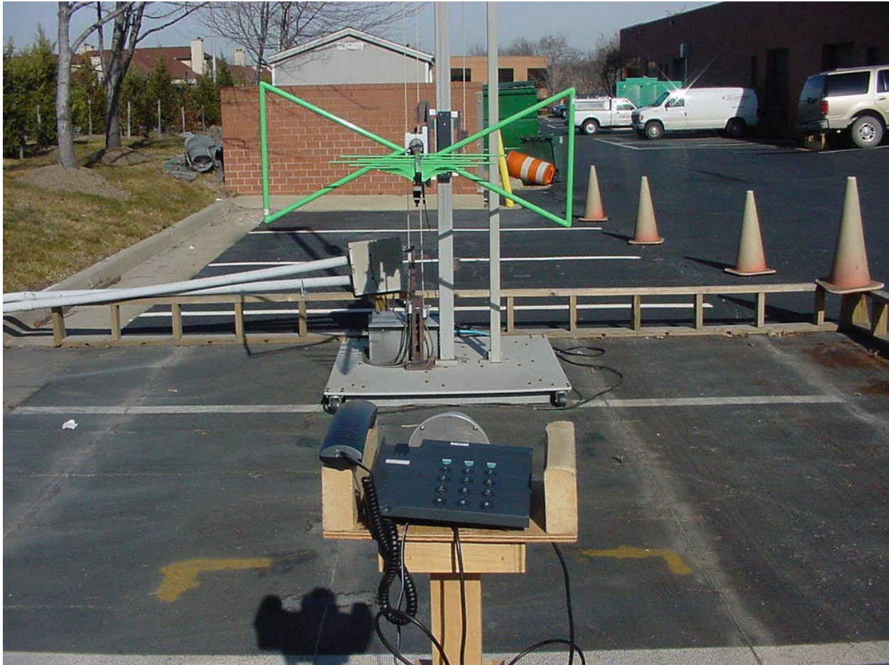
PHOTOGRAPH 4: RADIATED FRONT VIEW WITH PATCH ANTENNA
