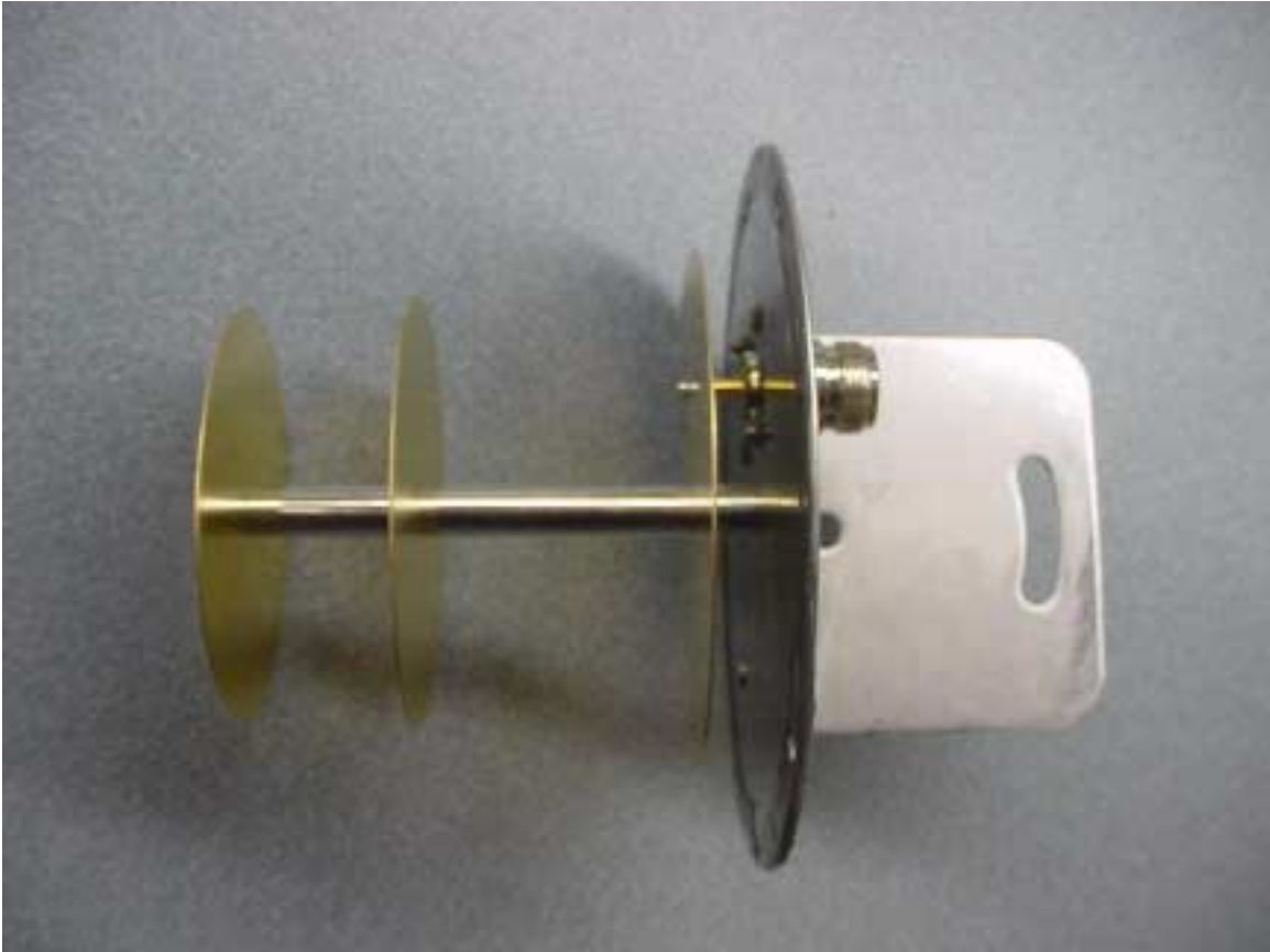
PHOTOGRAPH 40: INSIDE VIEW OF 10 DBI ANTENNA
