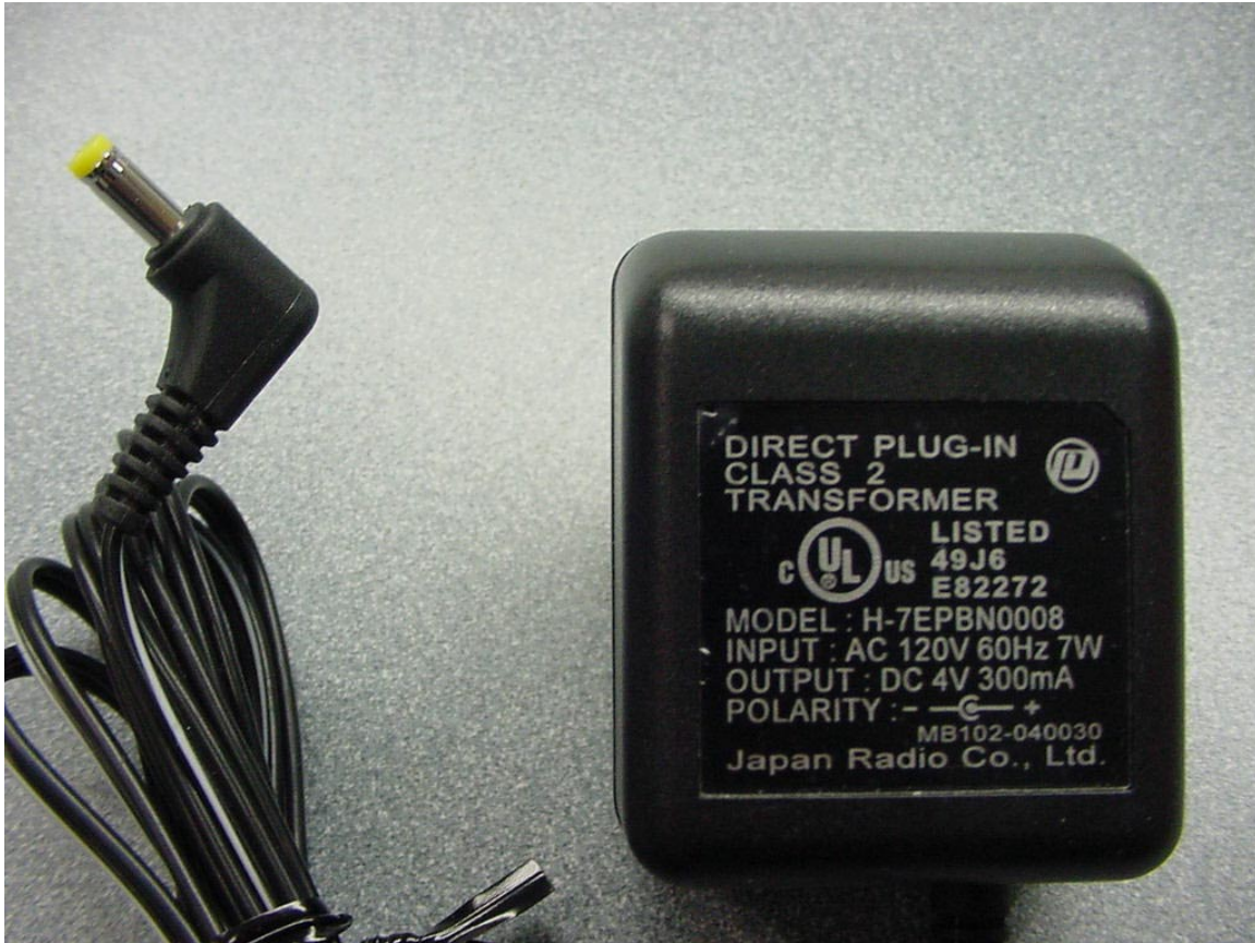
PHOTOGRAPH 12: 4VDC POWER SUPPLY
