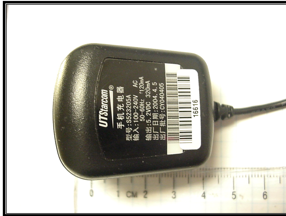
PHOTOGRAPH 13: TOP S523205A CHARGER
