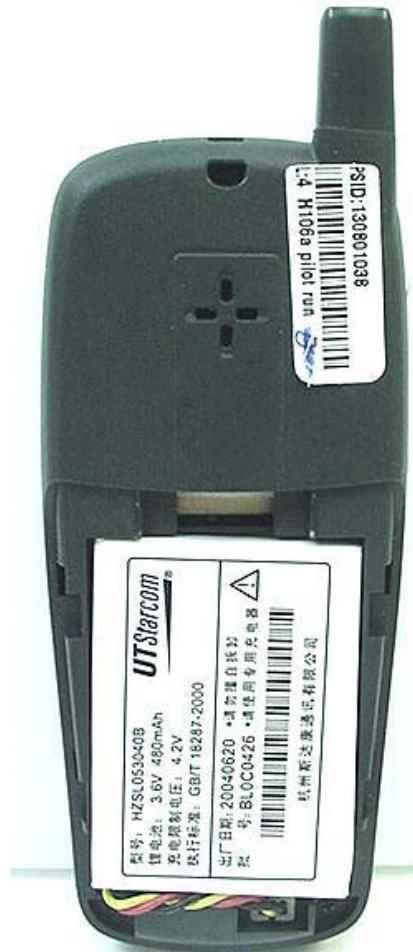
Li-ion Battery in DUT
