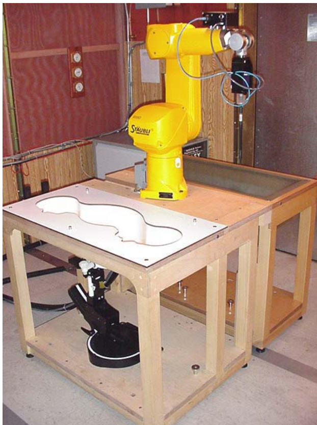
DASY4 Measurement System with SAM Phantom
