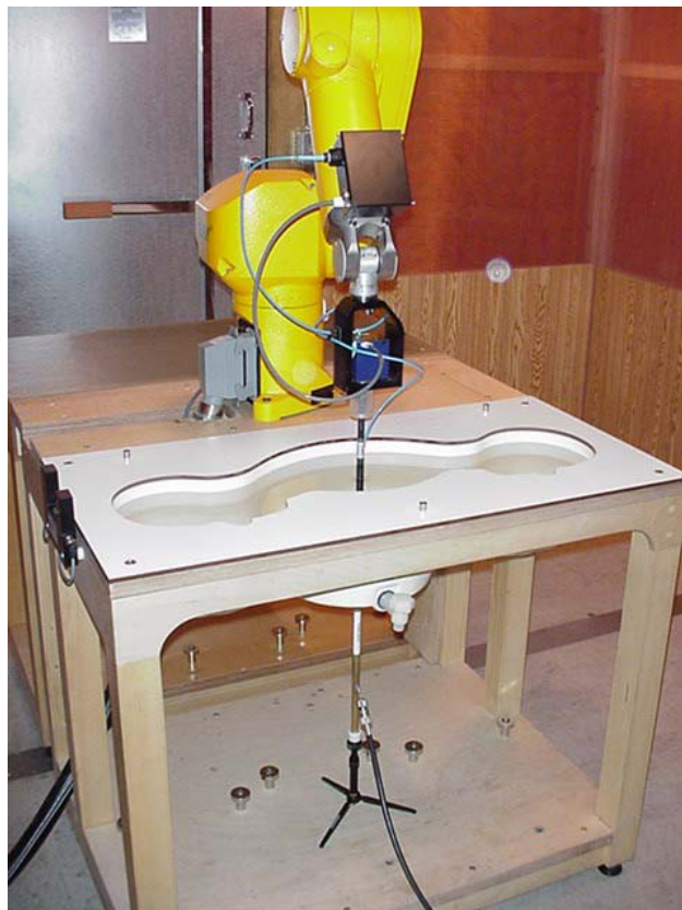
DASY4 Measurement System with SAM Phantom
